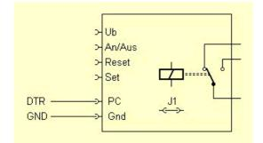
With a mixed use of pushbutton- and PC-controlled inputs you can exploit the priority of the SET ür RESETinputs. With the pushbuttons you can switch ON and OFF, but the "PC"-input can at any force a load to be swiched off over the RESET-input.
