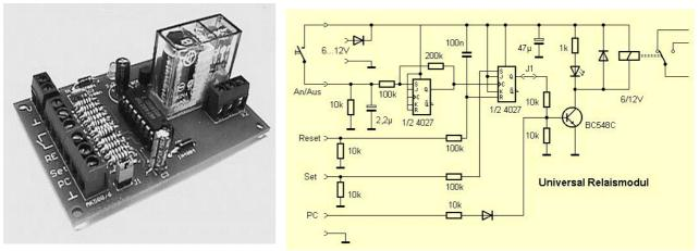
Usable as Latching- ("Toggle"), Set/Reset- or computer-controlled relay and many more. For 12V- or 6V-relays with 2x changeover-contacts (DPDT)
