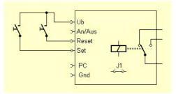
For direct PC-control or for control from other hardware you can use the "PC"-Input. A DC-voltage of +5V or more switches the relay to ON-state. A pull-down resistor at the base of T1 keeps the relay in the OFFstate when no DC-voltage is present.
