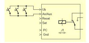
In addition (or as an alternative) you can connect pushbuttons for setting directly the ON- or OFFstate like it's utilized at motor-switches.
